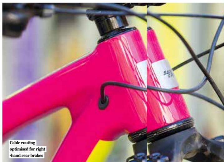
Cable routing optimised for right-hand rear brakes
